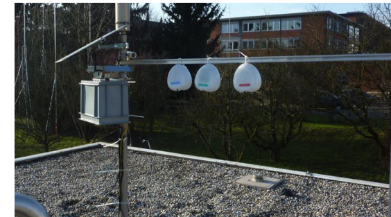
Low-cost devices for home deployment (calibration tests at the NABEL station in Dübendorf)
