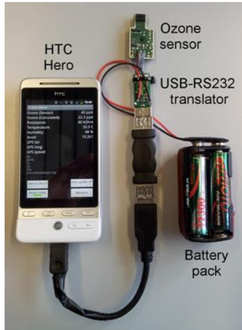
Smartphone connected to ozone sensor and various application software for Android
